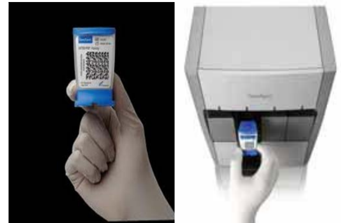
Figure 1: GeneXpert cartridge (left) and 4-module instrument (right)
